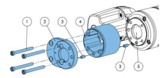
When ordering a VGP20 for Techman or Omron TM, the **Adapter K** plate (2) and **Extender flange** (4) will automatically be added to the Techman Robot Kit and Omron TM Robot Kit before shipment.
